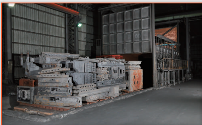
3 | 2門2台車式焼鈍炉 ( 9m×4m×4m ) x 1基 Double Door, Double Trolley Annealing Furnace ( 9 m x 4 m x 4 m ) x 1 set
