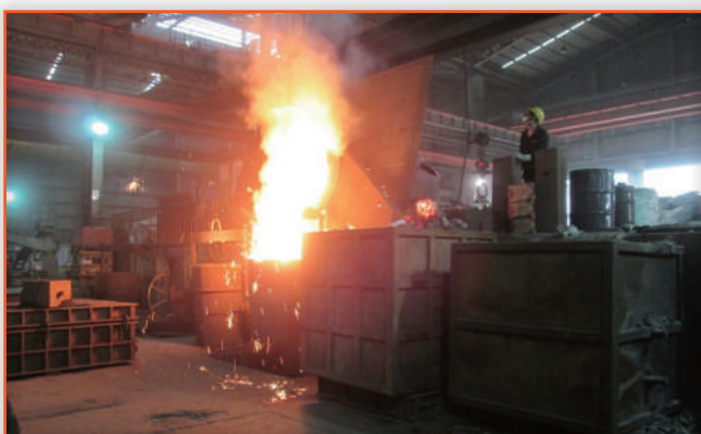
2 | 中周波感应電炉 ( 5T ) x 2基 Five-ton Medium Frequency Induction Furnace x 2 sets
